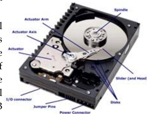
Fig 3.4: Internal View of Hard disk Drive
