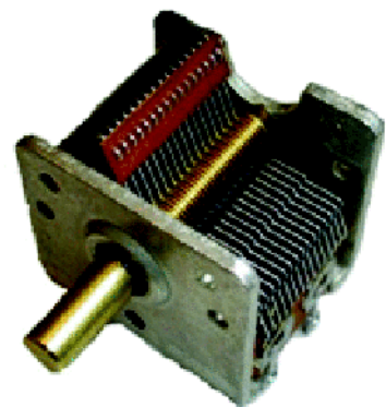
Fig 1.19 Air-gang capacitor (variable)
