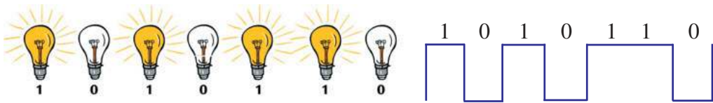
Fig. 1.8 : Digital representation of ON and OFF states
