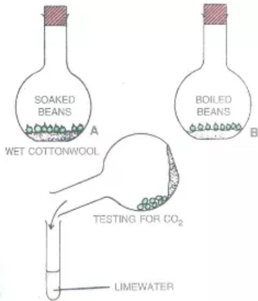
Experiment to show that germinating seeds produce carbon dioxide
