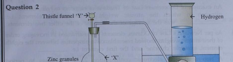
The apparatus above is set to obtain hydrogen gas in the laboratory
