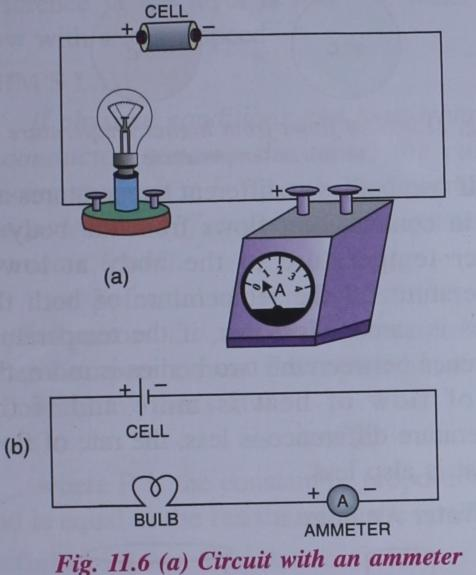
(b) Circuit diagram with an ammeter
