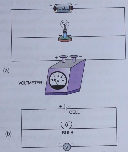
Fig. 11.8 (a) A circuit in parallel with voltmeter (b) Circuit diagram with a voltmeter
