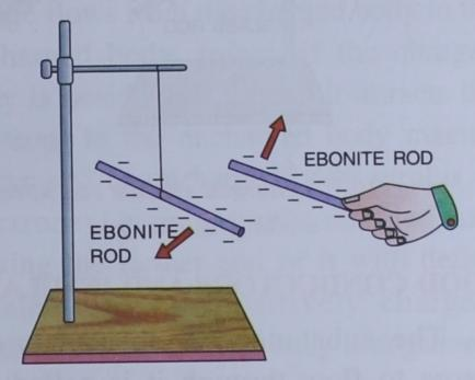
Fig. 10.6 Two charged ebonite rods repel each other
