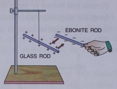
Fig. 10.7 A charged ebonite rod attracts a charged glass rod
