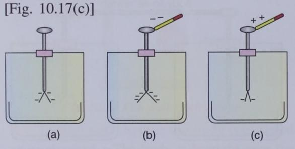
Fig. 10.17 (a) Negatively charged electroscope, (b) Body is negatively charged,
