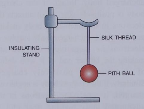
Fig. 10.10 Pith ball electroscope
