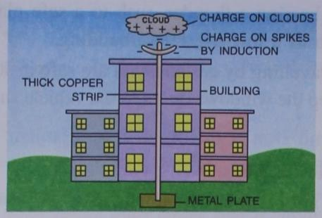
Fig. 10.19 Lightning conductor
