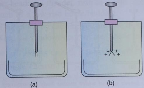
Fig. 10.14 (a) Uncharged electroscope and (b) Charged electroscope
