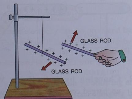
Fig. 10.5 Two charged glass rods repel each other
