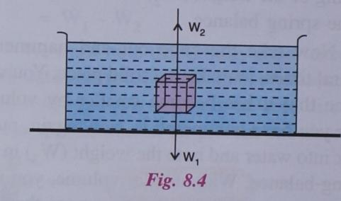
(a) Weight of the body  $W_1$  acting vertically downwards passing through the centre of gravity of the body.
