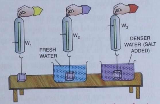
Fig. 8.2 Denser the liquid, more is the upthrust
