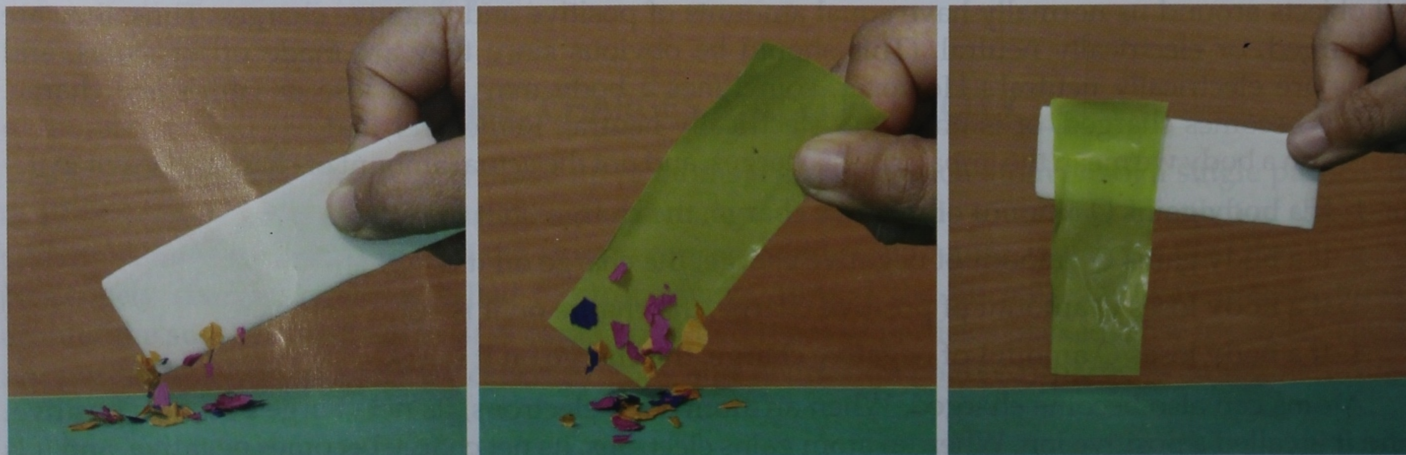
Fig. 6.4 The Styrofoam and polythene attract bits of paper. They also attract each other.
