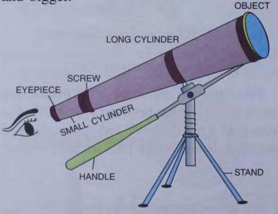
Fig. 4.6 A telescope
