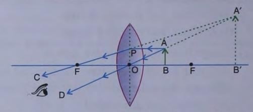
Fig. 4.2 Convex lens used as a magnifying glass
