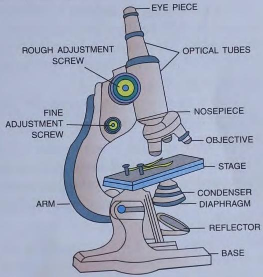
Fig. 4.4 A compound microscope
