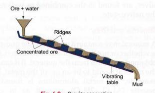
A special type **Driveling deer fitted Withs:// www.studiestoday.com** ridges, is generally used for gravity separation. A mixture of the ore and water is passed over the table, which is made to vibrate. The heavy ore particles are caught in the ridges and the muddy impurities are washed away.
