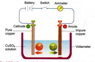
Fig. 6.12 The electrolysis of an aqueous solution of CuSO<sub>4</sub>, using copper electrodes
