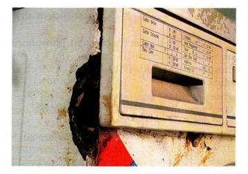
Taway from the sea. Fig. 6.7 Corrosion in the body of a washing machine Downloaded from https:// www.studiestoday.com
