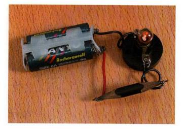
Fig. 6.5 Graphite conducts electricity.
