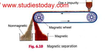
separating the nonmagnetic ore tinstone from its magnetic impurities.
