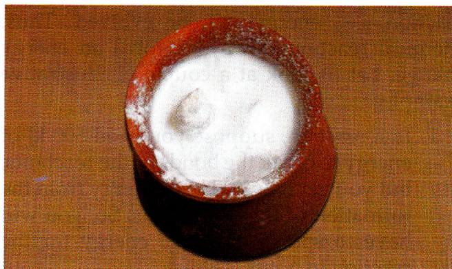
Fig. 5.10 The slaking of lime is a highly exothermic reaction.
