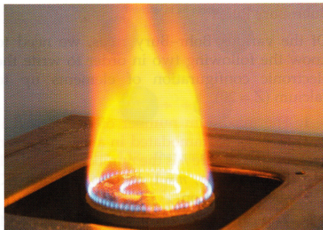
Fig. 4.10 Crystals of table salt impart a golden yellow colour to a blue flame due to electron transition in sodium.
