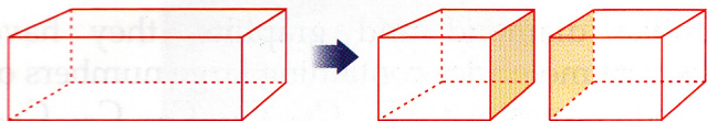
Fig. 2.9 The surface area of a solid increases on breaking. The shaded surfaces, not present in the original body, have appeared.
