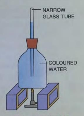
Fig. 4.17 Liquids expand on heating and contract on cooling
