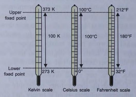
Fig. 4.7 Temperature scales of thermometers
