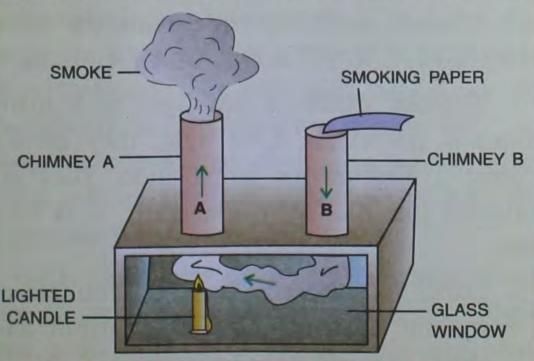
Fig. 4.23 An experiment to show convection in gases
