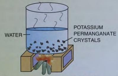
Fig. 4.22 An experiment to show convection in liquids
