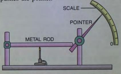
Fig. 4.10 Metals expand on heating
