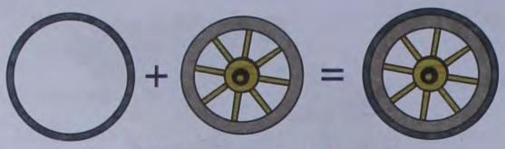
Fig. 4.15 An iron rim is heated to fit it on a wooden wheel
