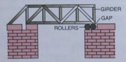
Fig. 4.12 Gap for the expansion in a bridge
