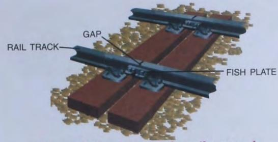
Fig. 4.13 Gap between the railway tracks
