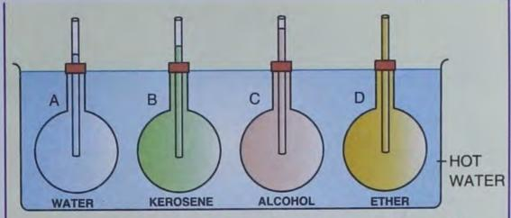
Fig. 4.18 Rates of expansion are different in different liquids
