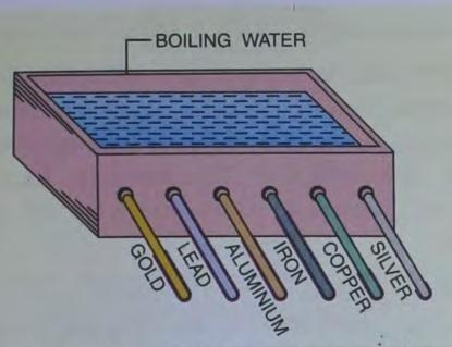
boiling hot water which heats the end of each rod in the trough to the same temperature. The heat starts flowing from the hot end to the cold end, where the match sticks have been fixed with the help of wax. As the temperature of the far ends reach the melting point of wax, the match sticks start dropping off. The match sticks on silver rod drops first showing that silver is the best conductor of heat followed by copper, gold, aluminium, iron and lead.
