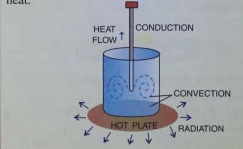
Fig. 4.19 An experiment to show how heat travels in different mediums
