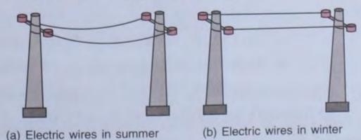
Fig. 4.14 Electric wires are kept loose for the contraction in winter
