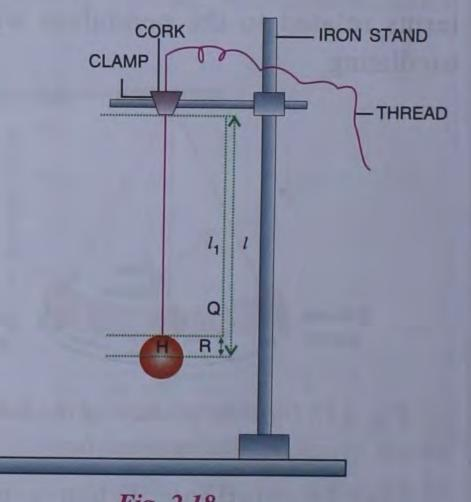
**Finding the time period of a simple pendulum Apparatus :** We need a metallic bob suspended by a strong but thin thread of about 100 cm in length; an iron clamp stand; a cork cut into two halves; a metre scale and a stop watch.
