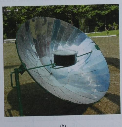
Fig. 6.15 Solar heaters use concave mirrors to concentrate the rays of the sun.
