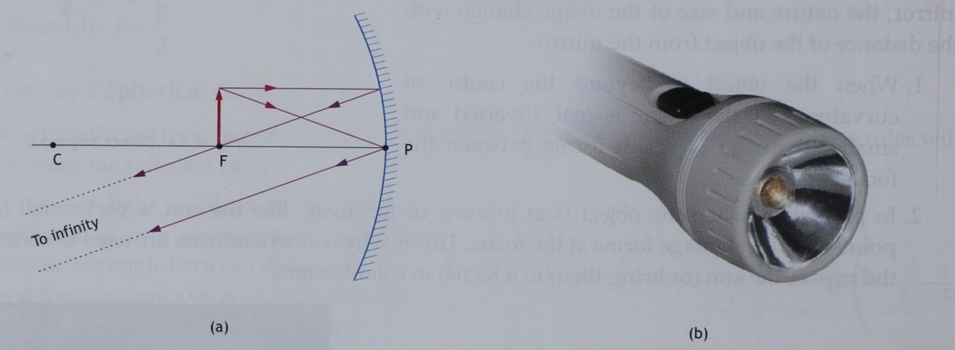
Fig. 6.18 The bulb is at the focus of the reflector in a torch, so the beam of light produced is almost parallel.
