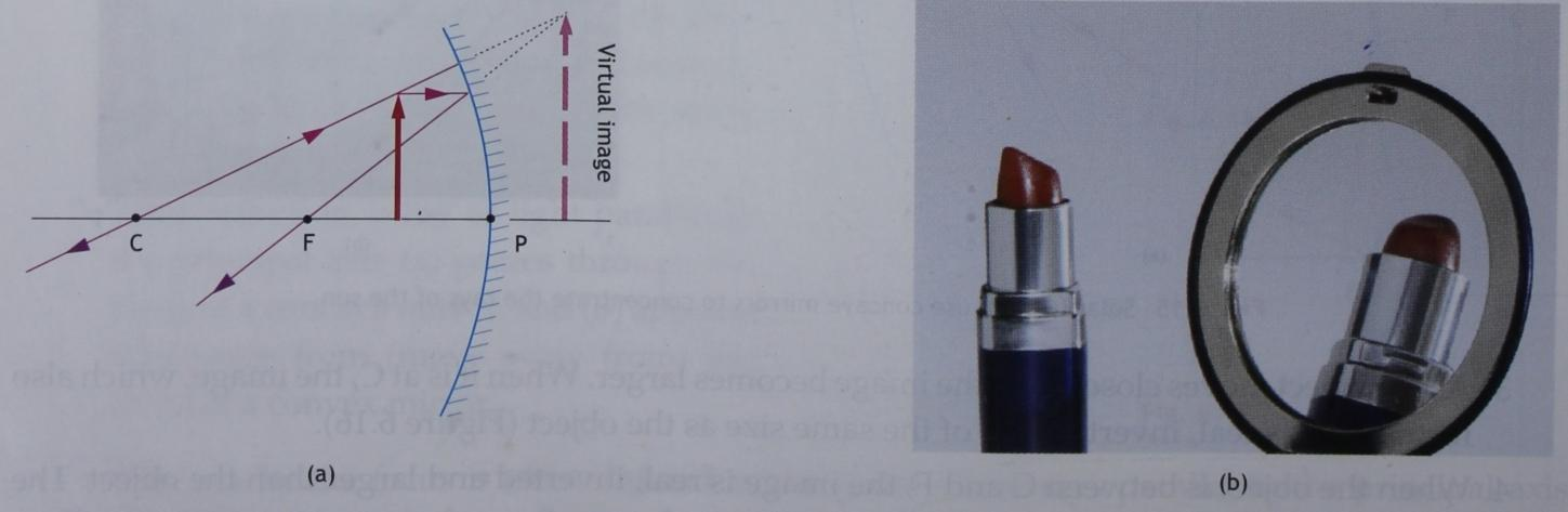
Fig. 6.19 Concave mirrors are used as 'shaving mirrors' or 'compact mirrors' because they produce a magnified image when held close to the face.
