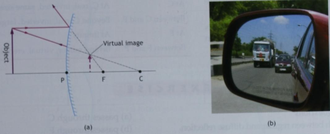
Fig. 6.20 (a) Convex mirrors produce images that are erect and smaller than the object.
