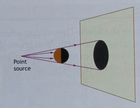
Fig. 5.9 A shadow formed by light from a point source is completely dark. It becomes larger as you move the screen farther away.
