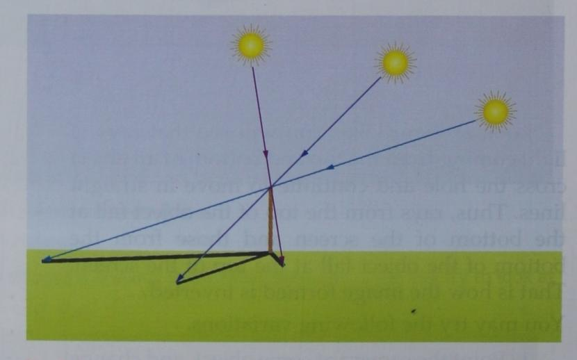
Fig. 5.8 The length of the shadow changes with the angle between the rays of the sun and the stick.
