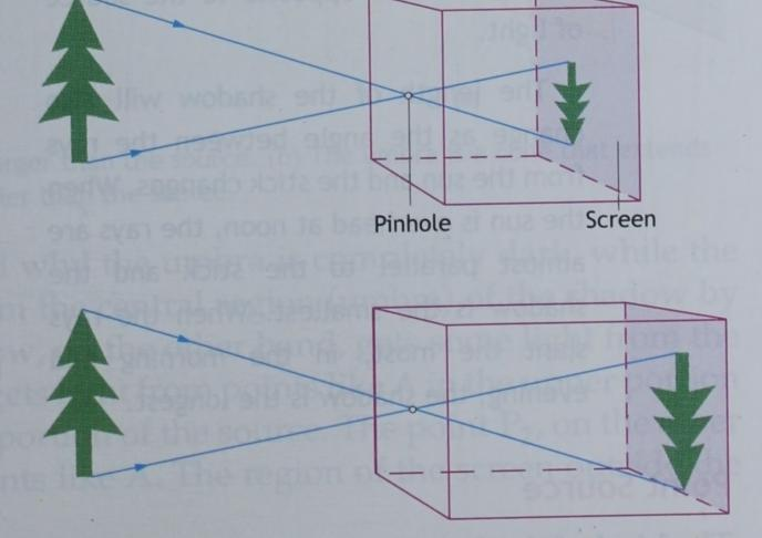
Fig. 5.6 The size of the image depends on the length of the camera.
