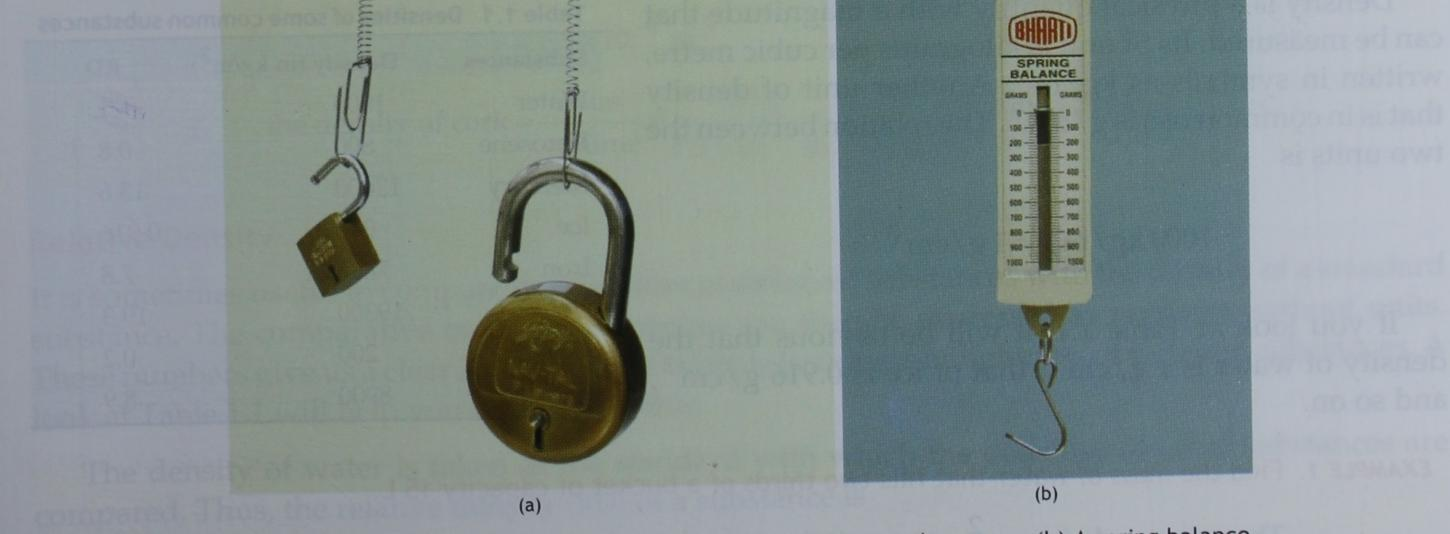
Fig. 1.3 (a) When you hang a heavier weight, the spring stretches more. (b) A spring balance works on this principle.
