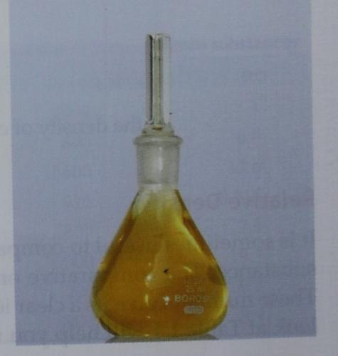
Fig. 1.4 Specific gravity bottle
