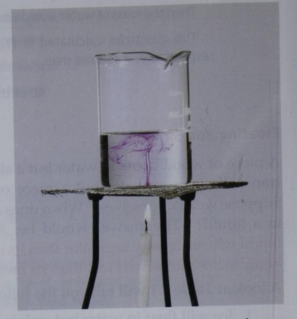
Fig. 1.6 Convection current in a beaker of water
