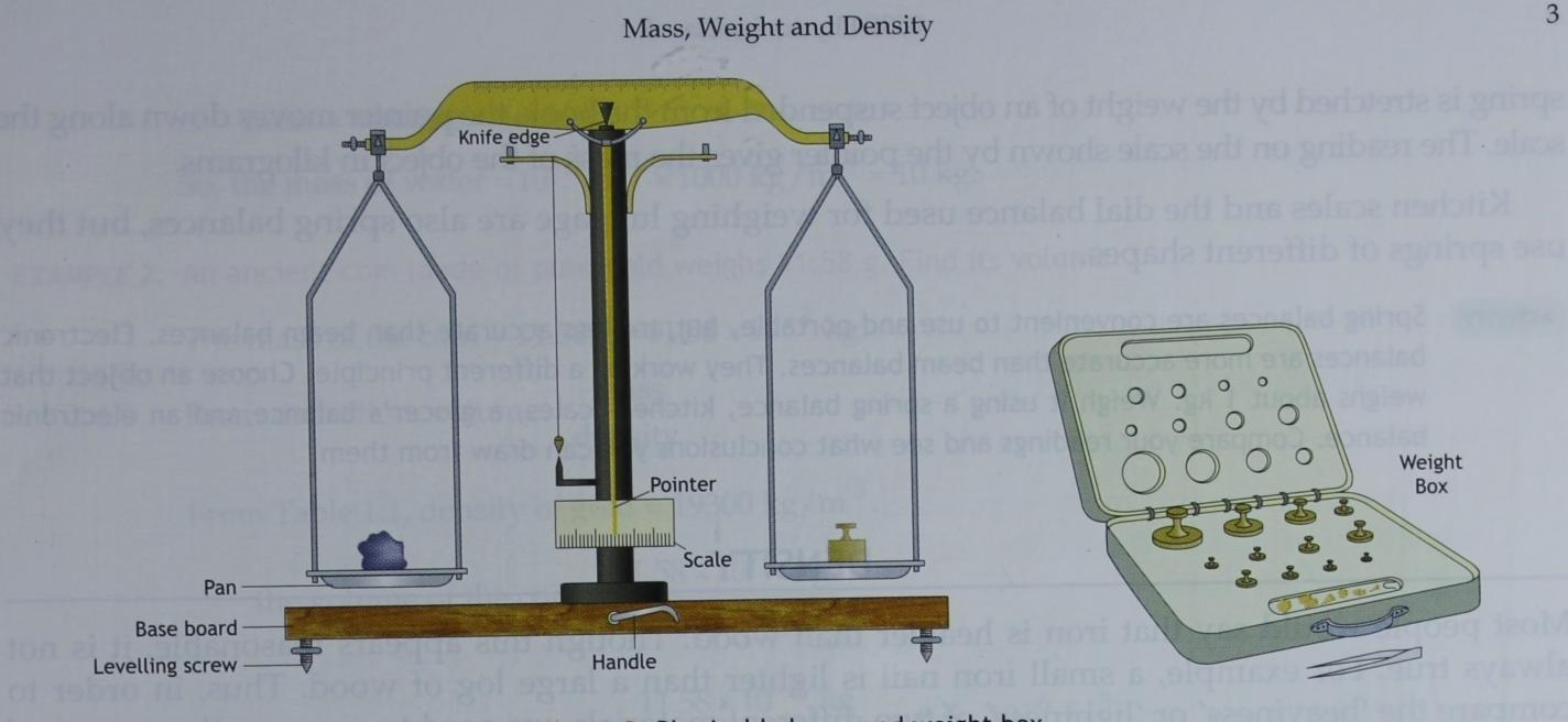
Fig. 1.2 Physical balance and weight box
