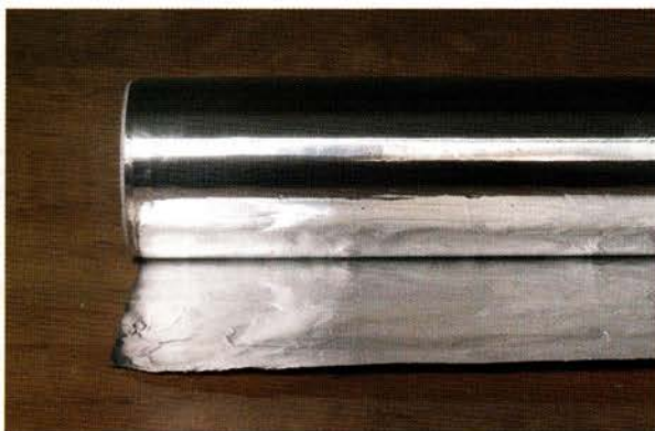
Fig. 6.2 Metals are ductile and malleable—they can be drawn into wires or pressed to form sheets or foils.
