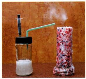
To make a fire extinguisher, you would need a jar with a plastic cap (about the size of a 50-g coffee jar), a 2-mL disposable syringe, a drinking straw that bends at the neck, baking soda and hydrochloric acid upof head bath from https://www.studiestoday.com
