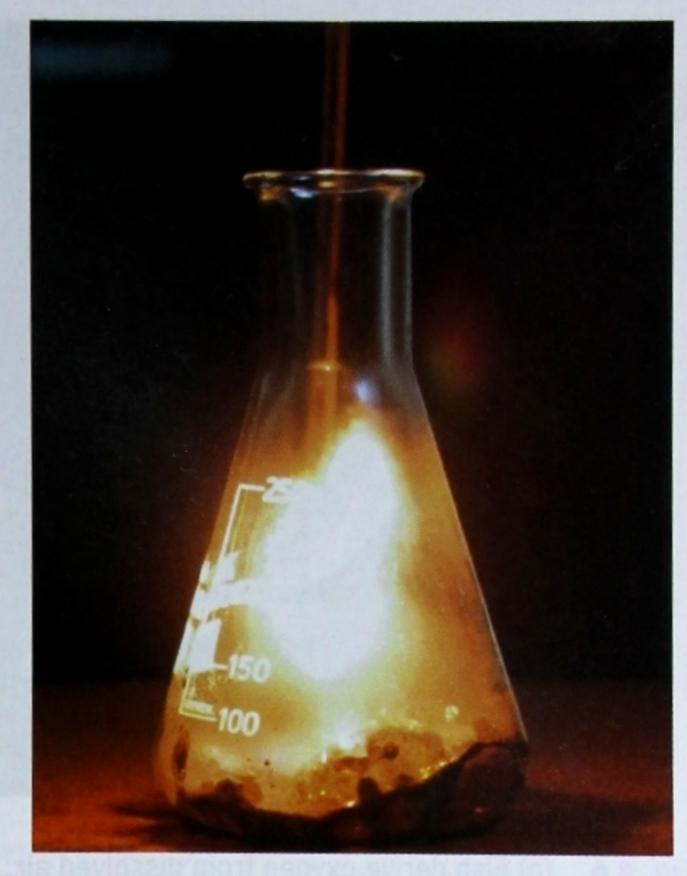
Fig. 4.5 A glowing splinter burns brightly in oxygen.
