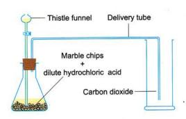
Fig. 4.9 Preparation of carbon dioxide
