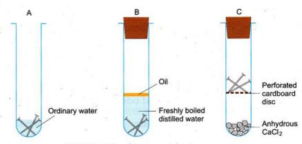
Fig. 4.3 Only moist air causes rusting. Rust on a nail Fig. 4.2 Downloaded from https://www.studiestoday.com
