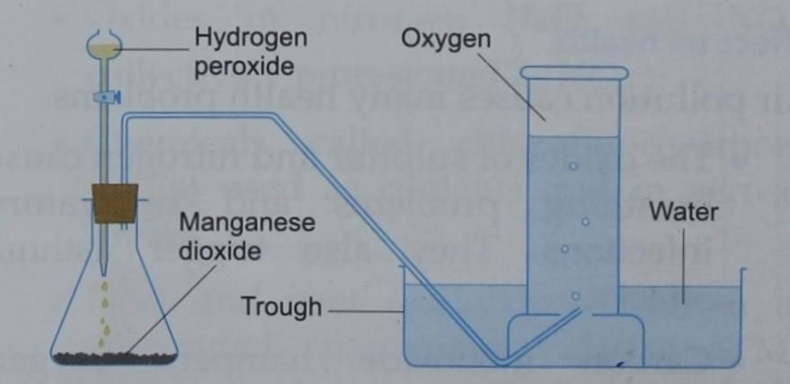
Fig. 4.1 The preparation of oxygen
