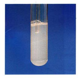
Fig. 4.11 Carbon dioxide turns limewater milky.
