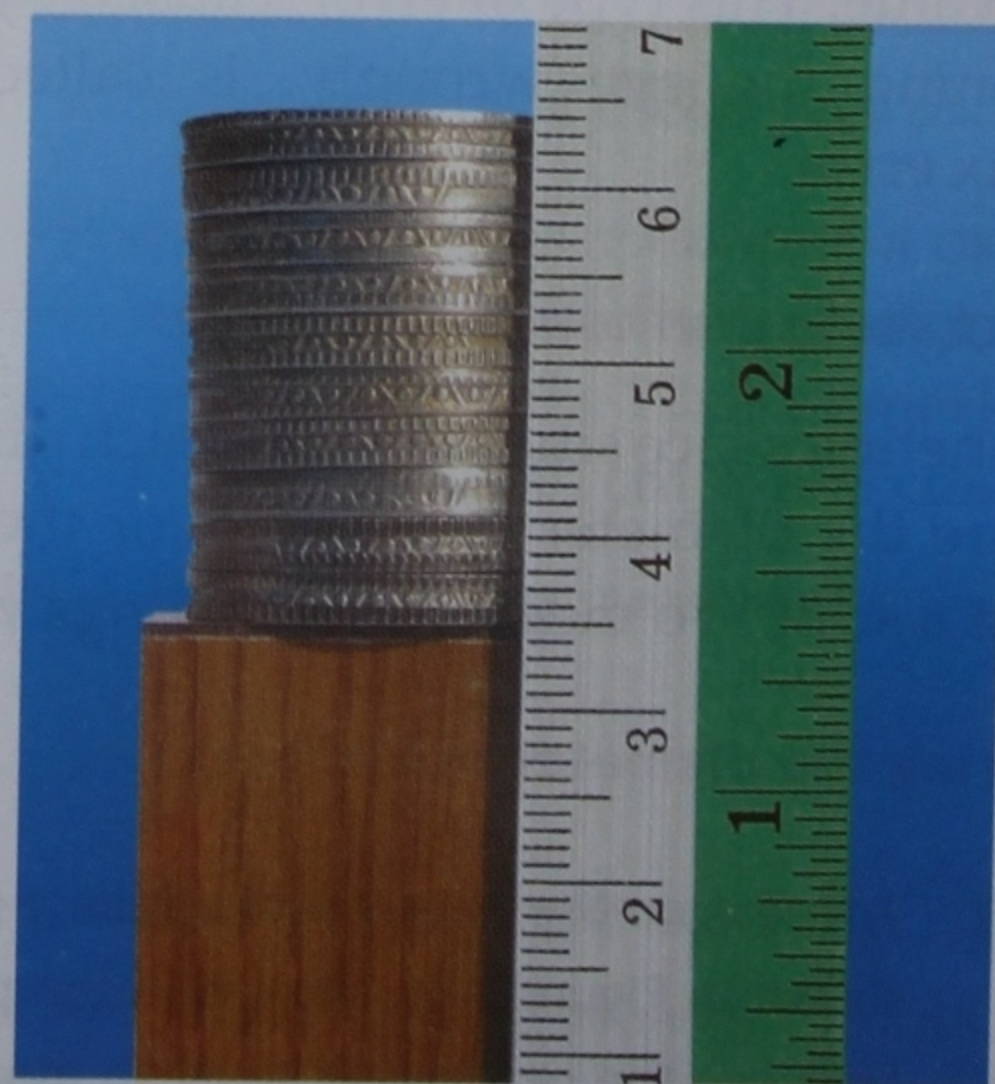
Fig. 2.8 Measuring the thickness of a coin
