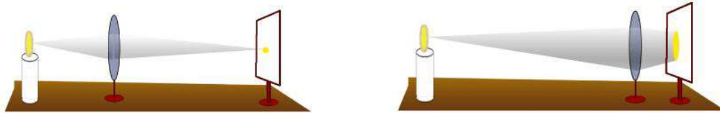
Fig. 12.20 Image formed by a convex lens for the candle flame placed at different distance from it.
